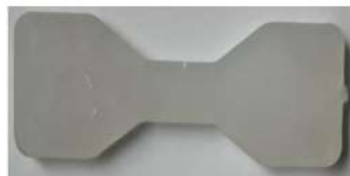
Fig. 2. Standard tensile test specimen
