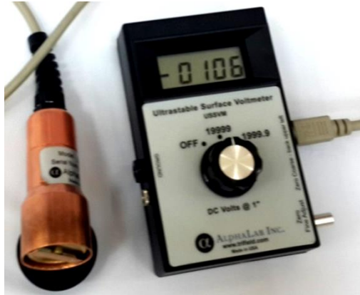
Fig. 1 Electrostatic field measuring device.
