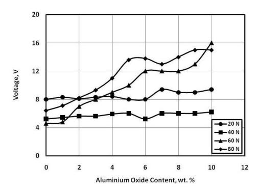
Fig. 22 Voltage generated from epoxy composites sliding against sand contaminating water/oil emulsion lubricated rubber.
