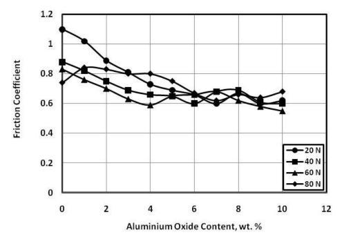
Fig. 11 Friction coefficient of epoxy composites sliding against oil lubricated rubber.
