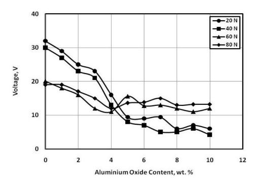
Fig. 20 Voltage generated from epoxy composites sliding against sand contaminating oil lubricated rubber.
