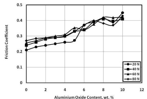
Fig. 17 Friction coefficient of epoxy composites sliding against sand contaminating water wetted rubber.
