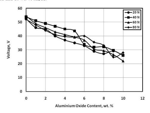
Fig. 24 Voltage generated from epoxy composites sliding against sand contaminating detergent wetted rubber.
