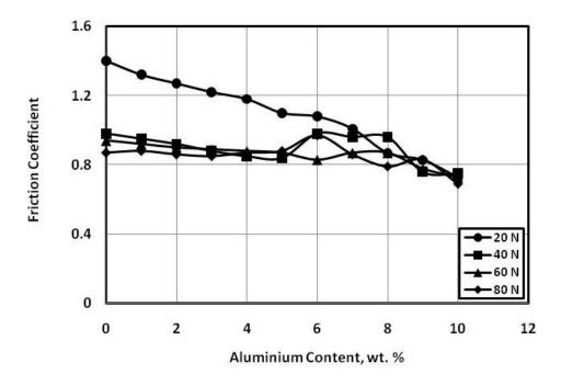
Fig. 5 Friction coefficient of dry sliding of epoxy composites against rubber.
