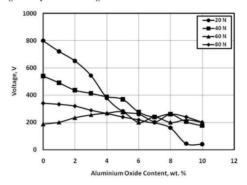
Fig. 6 Voltage generated from dry sliding of epoxy composites against rubber.
