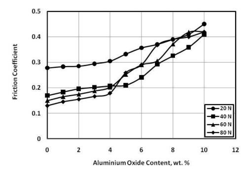
Fig. 21 Friction coefficient of epoxy composites sliding against sand contaminating water/oil emulsion lubricated rubber.
