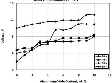
Fig. 16 Voltage generated from epoxy composites sliding against sand contaminated rubber.
