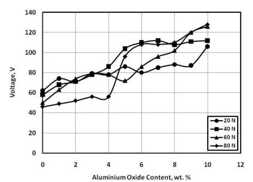
Fig. 18 Voltage generated from epoxy composites sliding against sand contaminating water wetted rubber.
