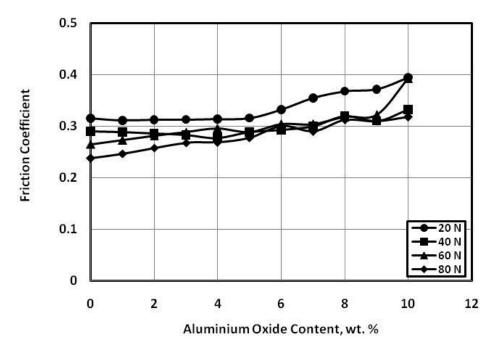
Fig. 23 Friction coefficient of epoxy composites sliding against sand contaminating detergent wetted rubber.
