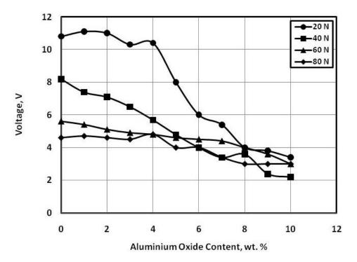
Fig. 14 Voltage generated from epoxy composites sliding against water/oil emulsion lubricated rubber.
