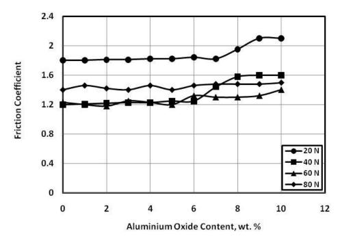
Fig. 9 Friction coefficient of epoxy composites sliding against detergent wetted rubber.
