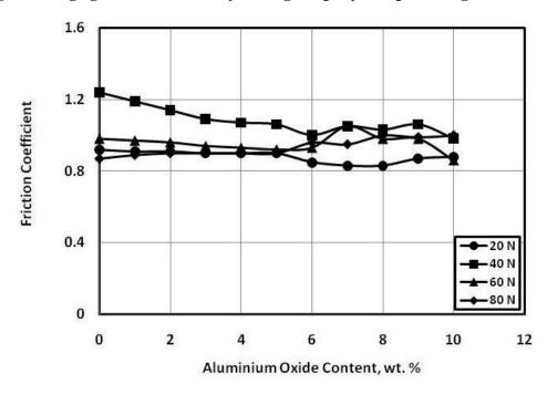
Fig. 7 Friction coefficient of epoxy composites sliding against water wetted rubber.
