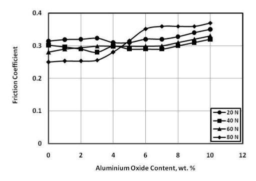
Fig. 15 Friction coefficient of epoxy composites sliding against sand contaminated rubber.
