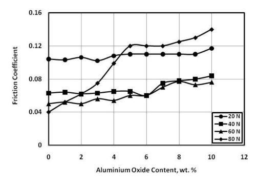
Fig. 13 Friction coefficient of epoxy composites sliding against water/oil emulsion lubricated rubber.
