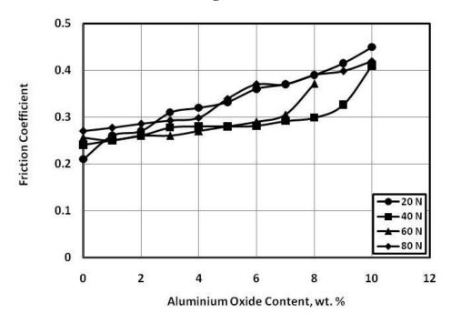
Fig. 19 Friction coefficient of epoxy composites sliding against sand contaminating oil lubricated rubber.
