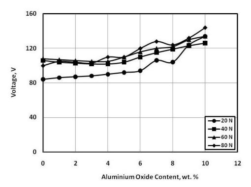
Fig. 10 Voltage generated from epoxy composites sliding against detergent wetted rubber.
