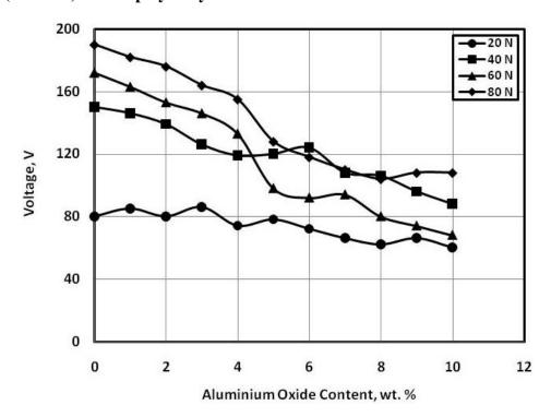
Fig. 12 Voltage generated from epoxy composites sliding against oil lubricated rubber.
