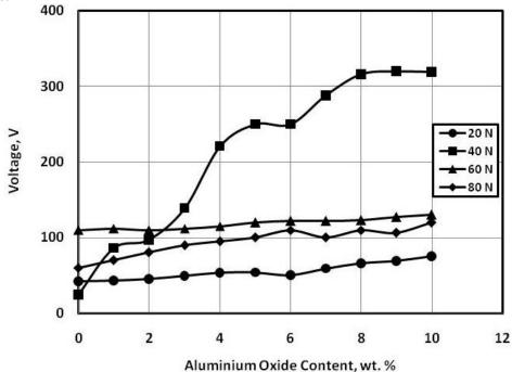
Fig. 8 Voltage generated from epoxy composites sliding against water wetted rubber.
