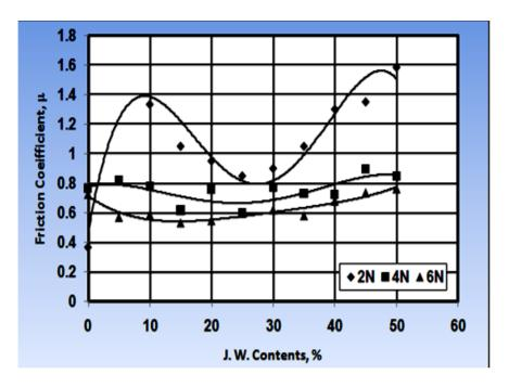
Fig. 4 Effects of coarse particles of jasmine leaves on the friction coefficient of polyester composite.
