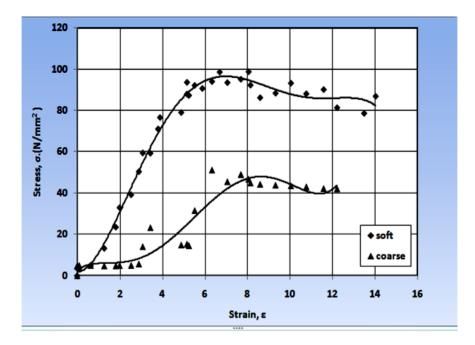
Fig. 8 Stress–strain curve for polyester composites filled by 30 wt. % jasmine. eaves.
