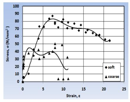
Fig. 9 Stress – strain curve for polyester composite filled by 50 wt. % jasmine leaves.
