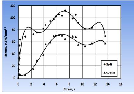
Fig. 7 Stress – strain curve for polyester composite filled by 5 wt. % jasmine leaves.
