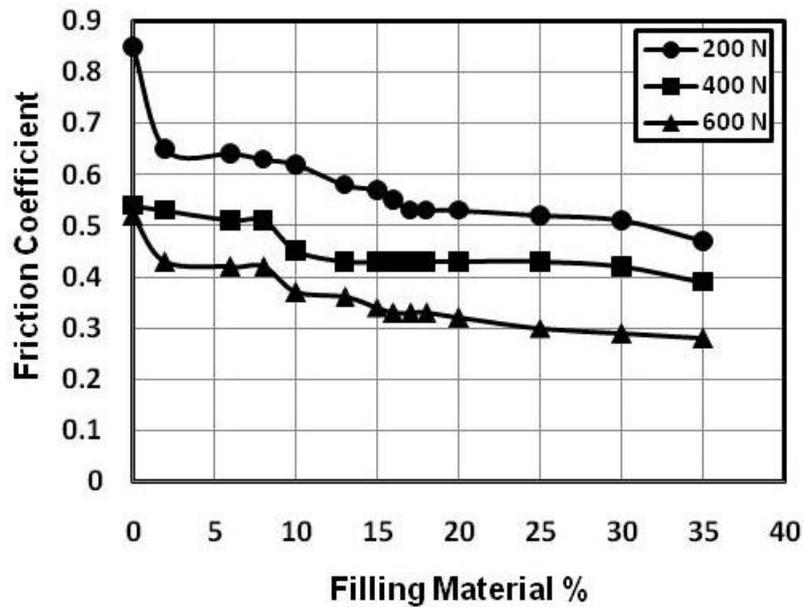
**Fig. 8 Friction coefficient of foot sliding against water lubricated flooring materials.**
