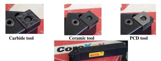
Tool holder Fig. 1 The three different tool materials with the tool holder.
