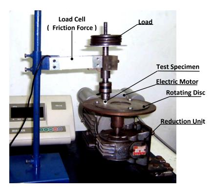
Fig. 1 Arrangement of the test rig.
