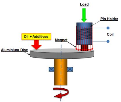
Fig. 2 Application of the magnetic field.
