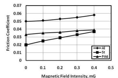
Fig. 4 Friction coefficient displayed by the sliding of steel pin against tested materials lubricated by oil dispersed by ZDDP.
