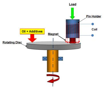
Fig. 2 Application of the magnetic field.
