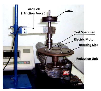
Fig. 1 Arrangement of the test rig.
