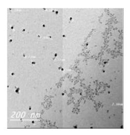
Fig. 5b. TEM image of the silver nanoparticles.
