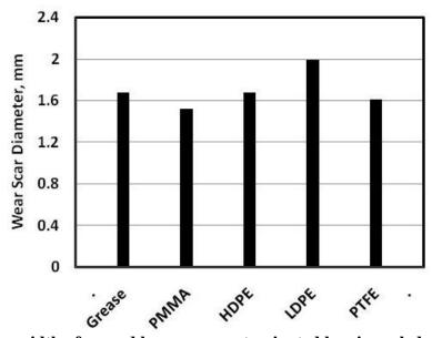
Fig. 4 Wear scar width of caused by grease contaminated by air cooled slag (high ferric particles).
