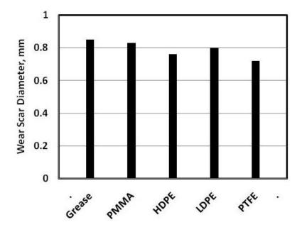
Fig. 2 Wear scar width caused by clean grease.
