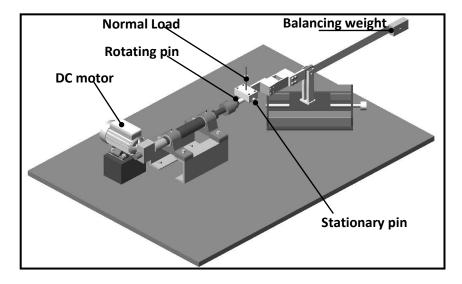
Fig. 1 Arrangement of the test rig.
