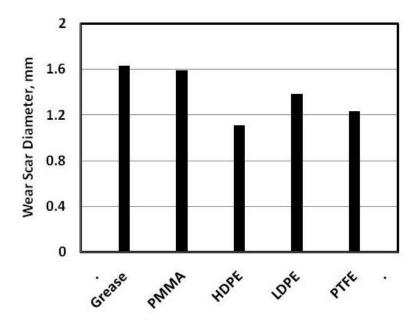
Fig. 9 Wear scar width caused by grease contaminated by water cooled slag (medium ferric particles).
