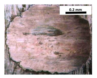
Fig. 10 Photomicrograph of the wear scar diameter caused by grease free of contaminants.
