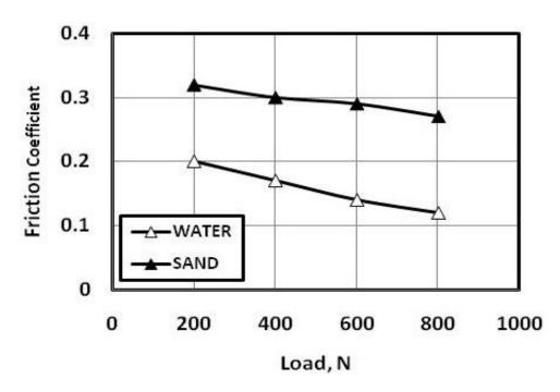
Fig. 6 Friction coefficient of water lubricated sliding of flat rubber against ceramic tiles.
