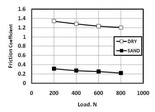
Fig. 5 Friction coefficient of dry sliding of rubber square protrusions against ceramic tiles.
