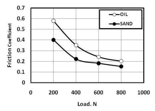
Fig. 13 Friction coefficient of oil lubricated sliding of rubber circular protrusions against ceramic tiles.
