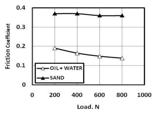
Fig. 15 Friction coefficient of oil and water lubricated sliding of flat rubber against ceramic tiles.
