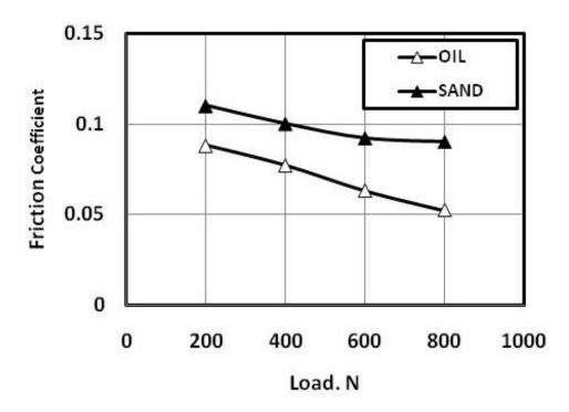
Fig. 12 Friction coefficient of oil lubricated sliding of flat rubber against ceramic tiles.
