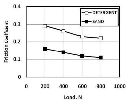
Fig. 11 Friction coefficient of detergent lubricated sliding of rubber square protrusions against ceramic tiles.
