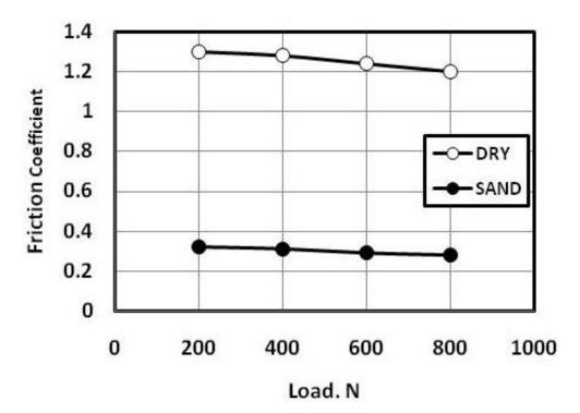
Fig. 4 Friction coefficient of dry sliding of rubber circular protrusions against ceramic tiles.
