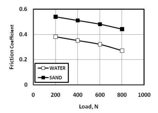
Fig. 8 Friction coefficient of water lubricated sliding of rubber square protrusions against ceramic tiles.
