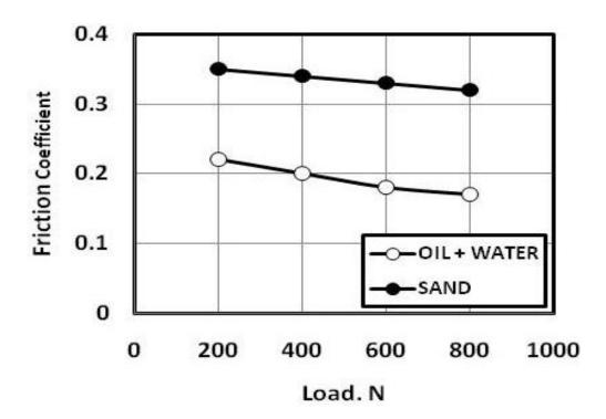
Fig. 16 Friction coefficient of oil and water lubricated sliding of rubber circular protrusions against ceramic tiles.
