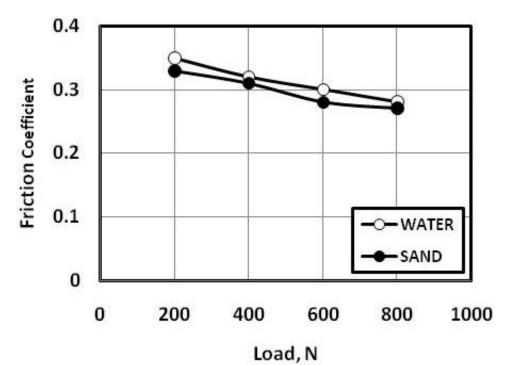
Fig. 7 Friction coefficient of water lubricated sliding of rubber circular protrusions against ceramic tiles.
