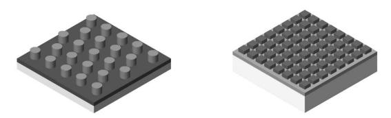
Fig. 2 Rubber test specimens of circular and square protrusions.
