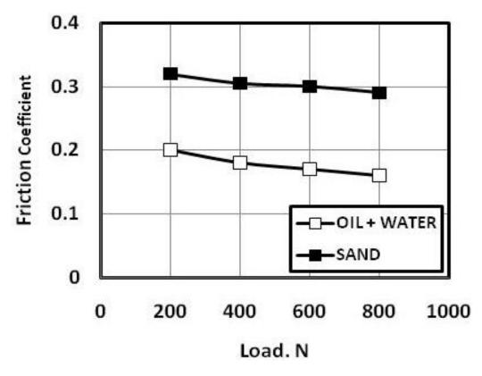
Fig. 17 Friction coefficient of oil and water lubricated sliding of rubber square protrusions against ceramic tiles.
