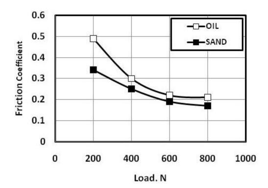
Fig. 14 Friction coefficient of oil lubricated sliding of rubber square protrusions against ceramic tiles.
