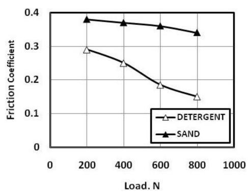
Fig. 9 Friction coefficient of detergent lubricated sliding of flat rubber against ceramic tiles.
