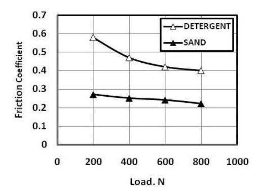
Fig. 10 Friction coefficient of detergent lubricated sliding of rubber circular protrusions against ceramic tiles.
