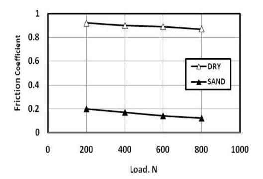
Fig. 3 Friction coefficient of dry sliding of flat rubber against ceramic tiles.
