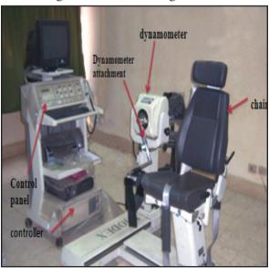
Figure (1): Biodex system 3 Isokinetic dynamometer.
