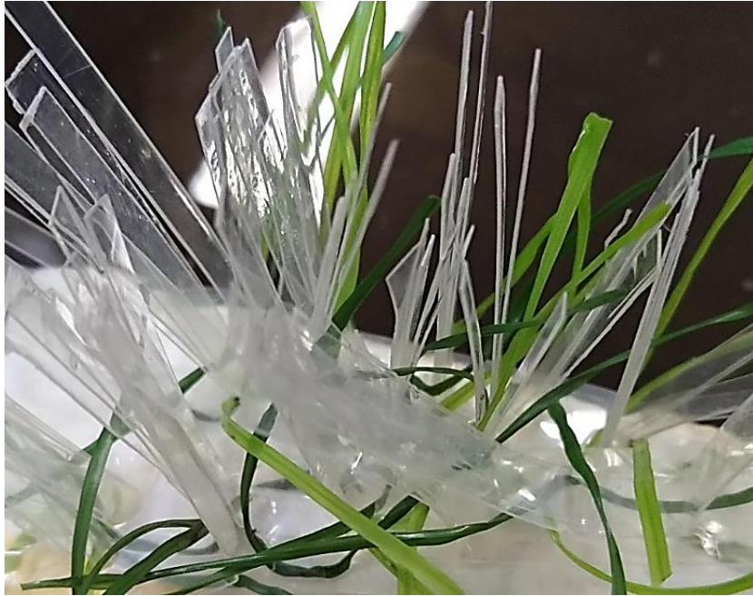
Fig. 2 PE blended by PU coated PP turf.
