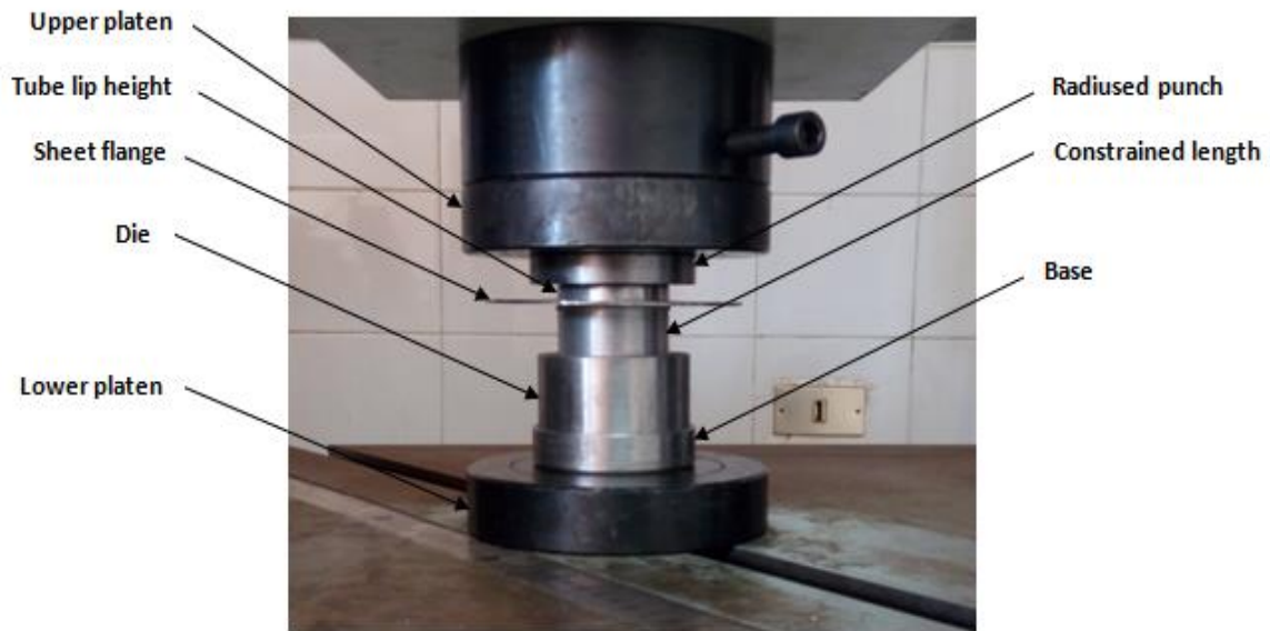
Fig. 7: Photograph of set-up joining attachment
