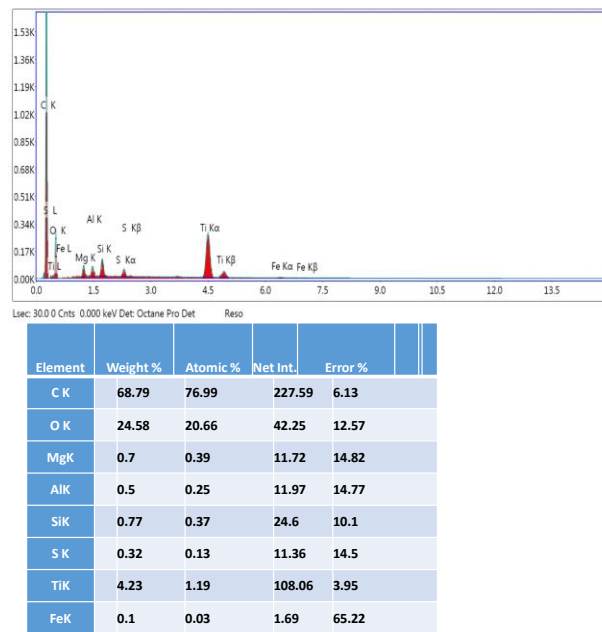
Fig.3 EDS elemental analysis of St. 304 sample coated with epoxy resin.
