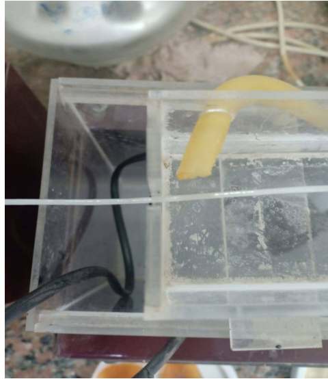
Figure 12: Filament cooling the water bath
