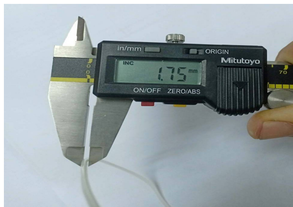
Figure 13 : Digital caliper verification filament from virgin HDPE pellets
