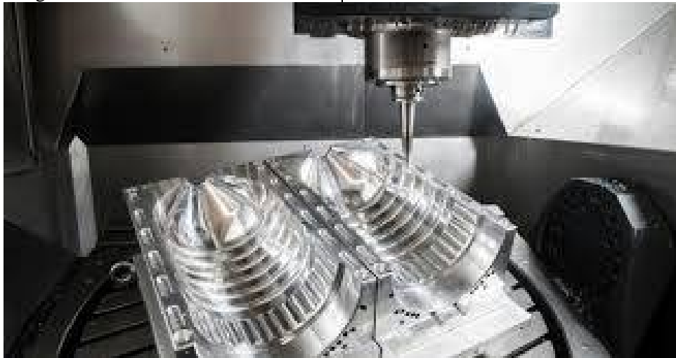
Figure 3: CNC milling metal blowing mold
