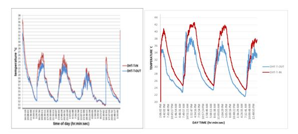
Fig. 12. Temperature in and out by using concrete trombe wall
