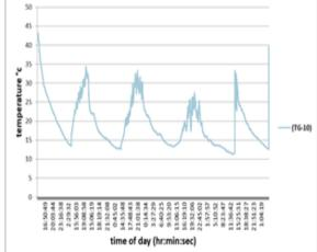
Fig. 16. The temperature of single glass of trombe wall
