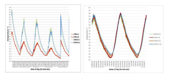
Fig. 14. temperature of mass wall of brick prototype trombe wall
