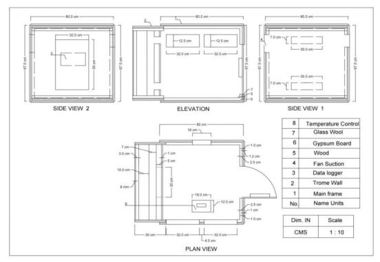
Fig. 1. Main assembly of the poultry house prototype
