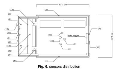
LDR – light sensor sensors ODSI8B20-temperature DHT22- temperature and humidity sensors
