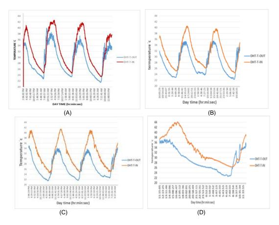
Fig. 18. The air temperature inside and outside the poultry house with different insulation
