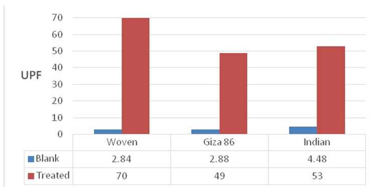
Figure 9 Effect of treatment application on Ultraviolet Protection Factor for the different types of cotton fabric The UPF results got better with treatment; the best UPF result was especially for the woven cotton fabric resulted from the presence of ZnO and the woven fabric structure, which is tight and provide better protection.
