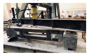
after each load increment up to failure. Dial gauges of 0.01 mm accuracy and total capacity of 20 mm were used for measuring deflections under the concentrated loads.
