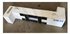
(b) Crack pattern for S30x12
