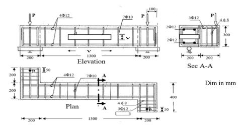
Fig. 2 : Dimensions and reinforcment details of refernce specimen with opening X\*Y
