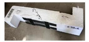
(a) Crack pattern for C30x6
