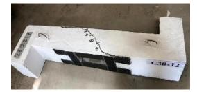
(b) Crack pattern for C30x12
