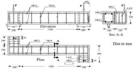
Fig. 1: Dimensions and reinforcment details of refernce specimen without opening R0
