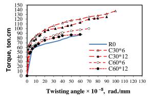
Fig. 18: Torque versus twisting angle for Group 5
