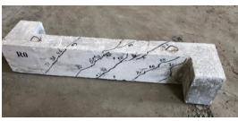
(a) Crack pattern for beam R0
