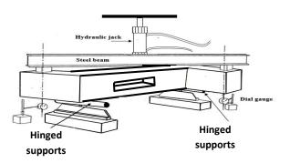
Fig. 7: Test set up and instrumentation
