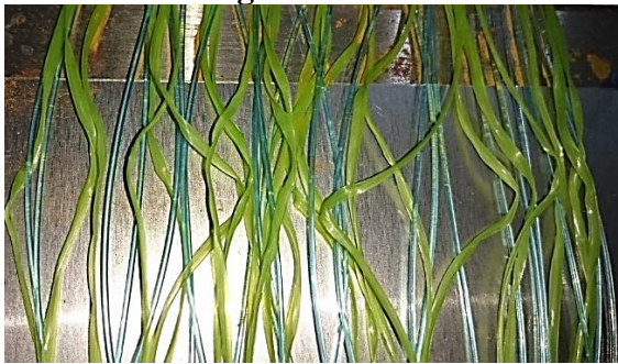
Fig. 5 PE blended by PA yarns of 0.3 mm diameter.
