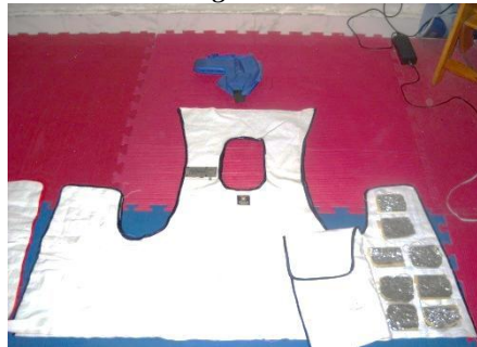
Fig. No. 3 shows real photos of the sensors between the uniform's layers
