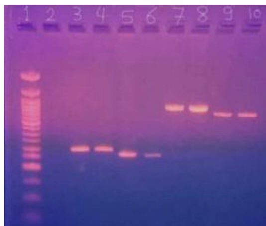
Figure (3): Agarose gel electrophoresis for the amplicons of different VacA subtypes: Lane 1 contains the DNA ladder (50 bp) and lane 2 contains negative control. While, lanes 9 and 10 contain the 570 bp VacA m1 gene, lanes 7 and 8 contain the 642 bp VacA m2 gene, lanes 5 and 6 contain the 259 bp VacA s1 gene and lanes 3 and 4 contain the 286 bp VacA S2 gene.
