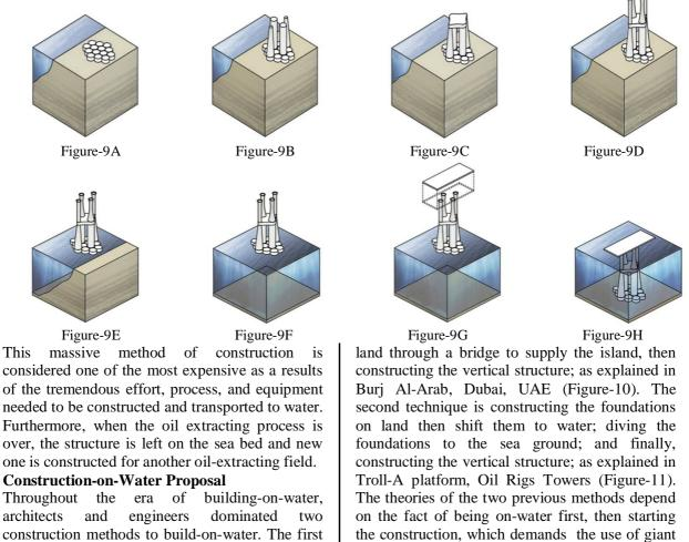
construction methods to build-on-water. The first technique, which is the most common, is building an artificial landfill island on the water, construct the foundation piles, connecting the island to the construction ships to transport heavy equipment, materials, and machineries to be on-water in order to be able to build the vertical structure.
