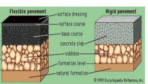
Fig(4): Comparison of Flexible Pavement, Rigid Pavement[5]
