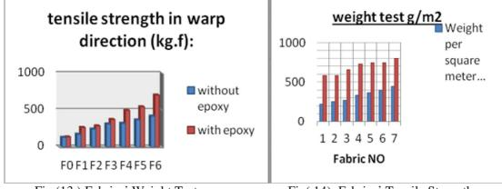
Fig (13):Fabrics' Weight Test By revising of the values in figure (13) it can be shown that sample F6 gave the highest tensile strength followed by F5 then F4, F3,F2, F1, F0 owing to glass yarn percentage on samples, By revising of the values in figure(14), it can be Fig(14) :Fabrics' Tensile Strength
