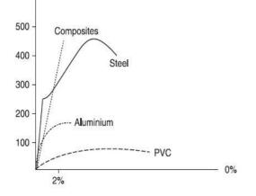
Fig(2):Glass-Fiber Reinforced Composite Rod Stress–Strain Curve (43) In reinforced concrete structures, ductility is
