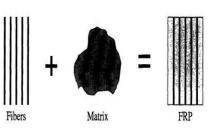
Fig(1): Formation of Fiber Reinforced Polymer Composite[3]
