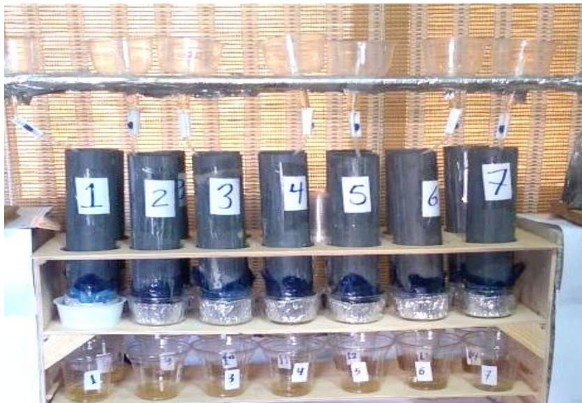
Fig. 2. Soil column experiments design incubated for 36 days with different rate of (OP) and (WC).
