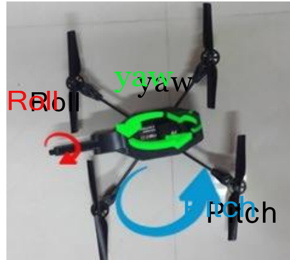
Figure 1: Roll, Pitch and Yaw
