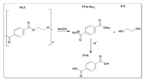
Scheme 3. Polyester chain alkaline hydrolysis mechanism [27].
