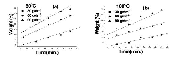
Fig. 5. Kinetic of weight loss % of polyester fabric treated with different concentrations of caustic soda at 80°C and 100°C.
