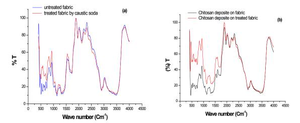
Fig. 4. FT-IR spectrum for untreated and treatedpolyester/ cotton blend fabric with (a) caustic soda[ C = 60 g/dm<sup>3</sup>, 100 °C,60 min] (b) chitosan[ 7 g/dm<sup>3</sup>, 25°C ,60 min].
