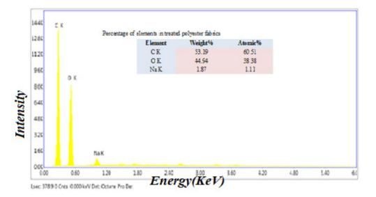
Fig. 3. EDX analysis of treated polyester fabric with caustic soda[C = 60 g/dm<sup>3</sup>,100 °C, 65min].
