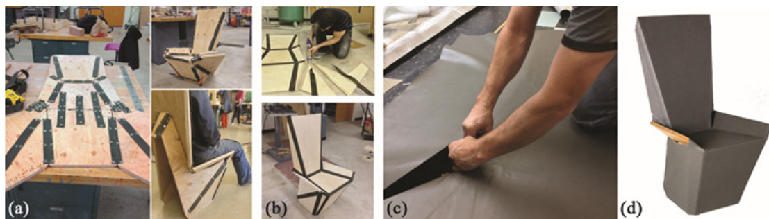
Figure 17: “Flat Stanley Origami Chair” designed by: Brett Mellor (a) Prototype. (b) Assembling (c) Covering with vinyl coating sheets (d) Final product (29) Accessed: 01/01/2020.
