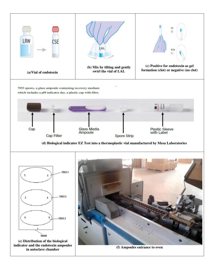
Plate I. Sterilization and depyrogenation tests
