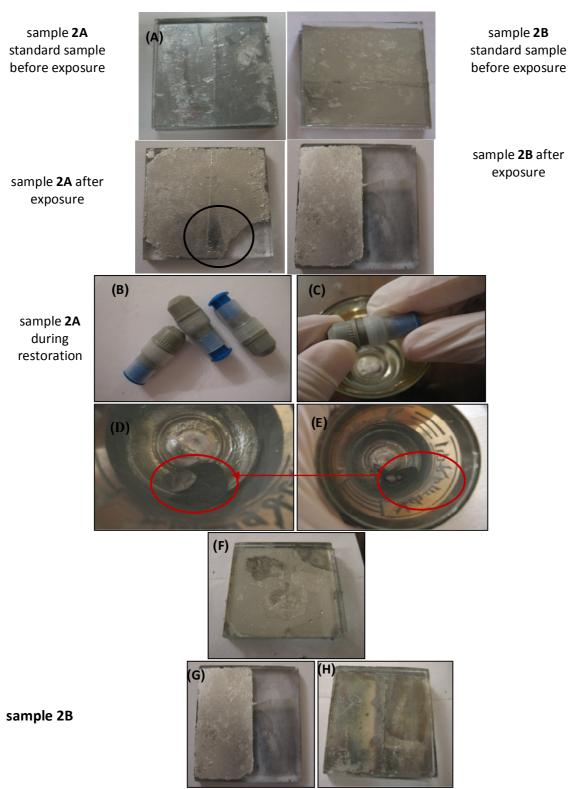
Fig.3. **Method of Partial Completion by dental amalgam** :A. Experimental sample that selected to be restored ;B. Teeth amalgamation tubes ;C. Opening teeth amalgamation tube to put powder in cup; D,E. Gradual increasing in the size of the mercury drop getting mixed with the powder even amalgamation occurrence.; F. Final form of the restored mirror with the dental amalgam.; G. the sample 2B before restoration. ; H. sample 2B after restoration.
