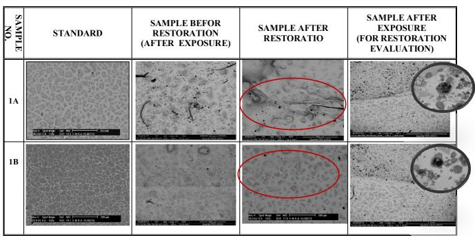
Fig.6.Evaluation of the restoration by the Method of Partial Completion with a new layer of tin and mercury (SEM microscope)
