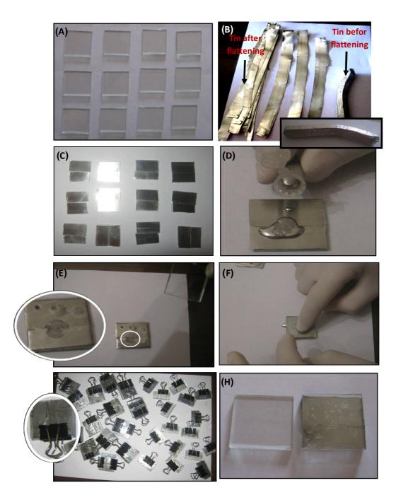
Fig.1.Preparation of experimental amalgam mirror samples :A. glass square samples have been prepared and cleaned;B. Tin rolling and flattening into longitudinal slices ;C.Placing the tin slices on the glass squares; D.Pouring liquid mercury on the tin; E.Darker spot appear once put the mercury on the tin; F.Press slowly the glass square after laying the glass on the mercury; G.Put clips for strong bonding; H.Square glass and resulting mirror.
