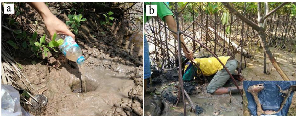
Fig. 3. Pouring the mixed liquid of polyester resin and hardener into in situ the burrow opening (a) and removing burrow casting from mud (b)
