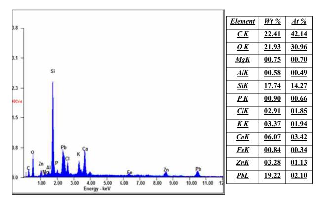
Fig. no. 4 Chart of the studied sample from the glaze layer by (EDX) of Terbana Mosque. KV: 30.00 Tilt: 0.00 Take-off: 35.00 AmpT: 102.4 Detector Type: SUTW-Sapphire Resolution: 129.66 Table No. 1 shows the elements by EDX Quantification & its concentration in the studied sample from the glaze layer of Terbana Mosque.
