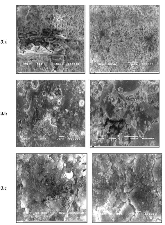
effect, i.e. flakes, cracks, crystallization in pores, and abrasion in some areas of the glaze (leading to exposure the tile body)<sup>15</sup>. Soluble salts either enter the clay body from the
