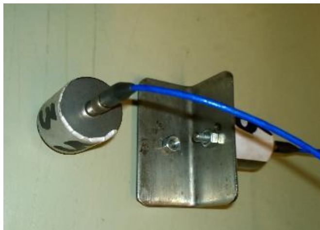
PCB accelerometers with magnetic mounting attached to the tower wall Figure (7) Test equipment
