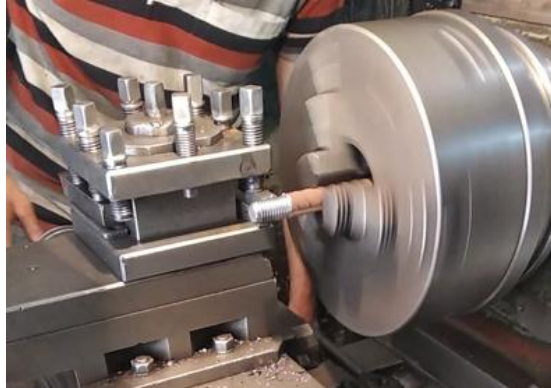
Figure 15: The process of threaded not enlarged rebar.
