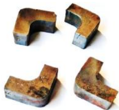
Fig 7: The shape of specimens after cutting process.
