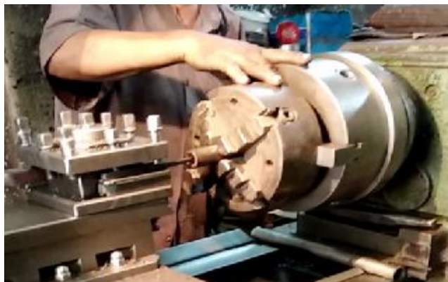
Figure 10: Process of internal threading using the lathe machine.
