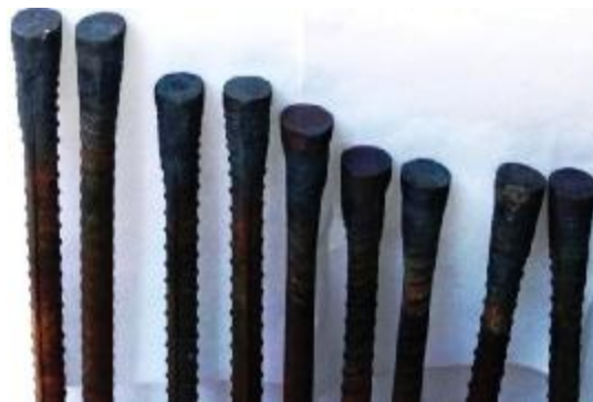
Figure 13: The reinforcing bars after enlargement process.
