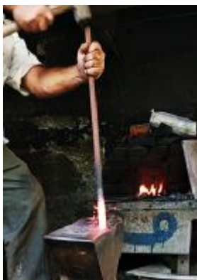
Figure 12: Knocking a heated reinforcing bar end.
