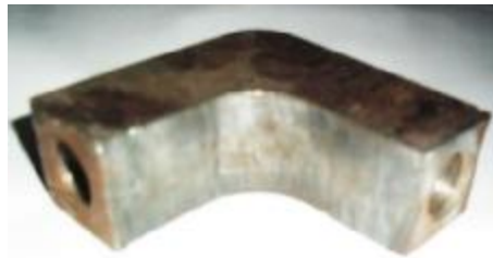
Figure 8: Two holes performed by Lath machine in the two coupler branches.
