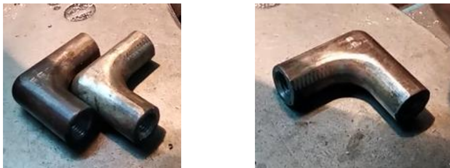
Figure 9: Shape of primary development of mechanical coupler.
