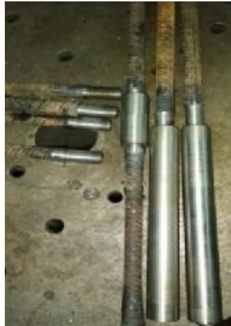
Figure 17: Couplers that connect one bar for each and a coupler connects two aligned bars.
