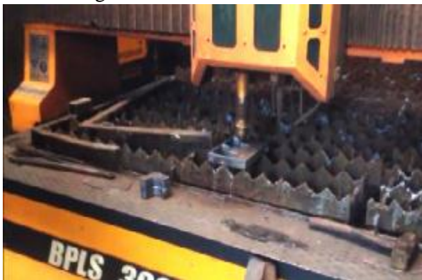
Figure 6 CNC plasma machine during cutting process.
