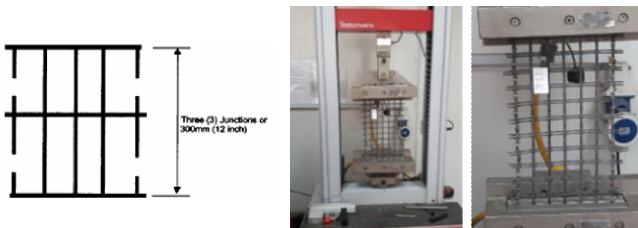
Fig. 2 Specimen configuration; Multi-Rib tensile method -ASTM D6637
