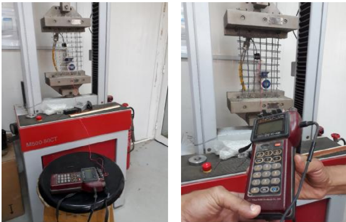
Fig. 8 CSR test setup adopted for derivation of CF
