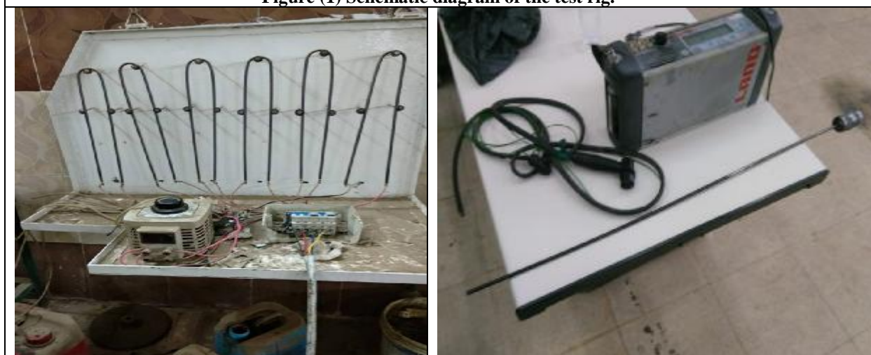
Figure (2) Load table of 6 heaters each of 1KW and a power variac. – Lancam gas analyzer
