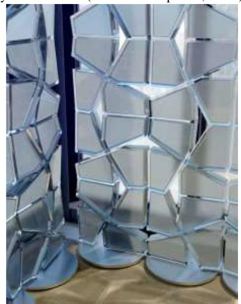
which is PCM material for storing latent heat and transparent aerogel units for thermal isolation.
