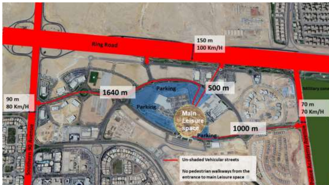
Figure (3) Cairo Festival City, New Cairo, Illustration shows the exclusion of the Leisure space due to being surrounded by fast vehicular streets and lack of pedestrian accessibility , (Map from Google Earth) (Illustration by researcher)
