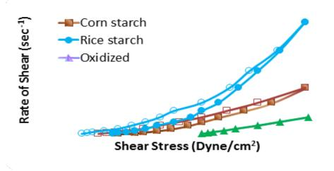
Fig. 3. Rheograms of freshly prepared starch formate derivatives after storing for 7 days.
