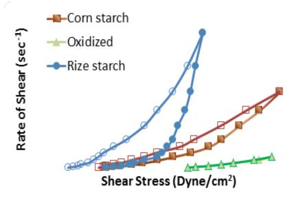
Fig. 2. Rheograms of freshly prepared starch formate derivatives after storing for 48 hours. Egypt. J. Chem. 61, No. 5 (2018)
