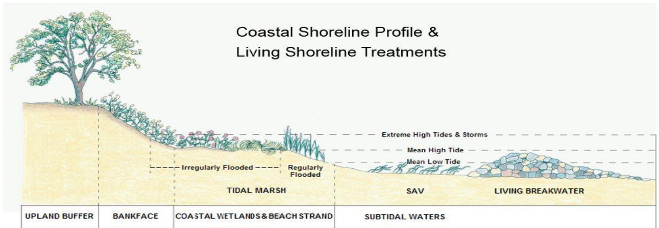
Figure (18). An illustration of the main concept of constructed wetlands for shoreline protection
