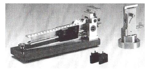
Fig. (2): Implement uses for determined the tensile force for breaking an individual fiber (Pressley – Code 231 A).
