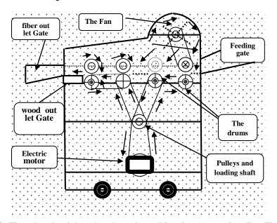
Fig. (1): The sketch of the developed machine for separation flax fiber
