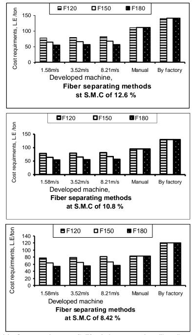
Fig. (7): Cost requirement (L.E/ton) for separating fiber flax under different parameters studies.
