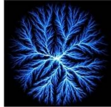
Fig. (6) Lichtenberg " lightning" formed by rapidly discharging electrons in Lucite.
