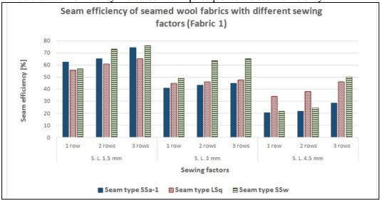
Figure 4: Seam efficiency of fabric 1 with different sewing factors**Determining the seam stiffness**measures seam stiffness is changing for allIt was observed from table 4 that with the repeatexperimental runs.
