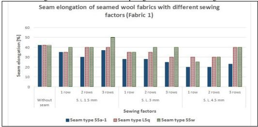
Figure 3: Seam elongation of fabric 1 with different sewing factors
