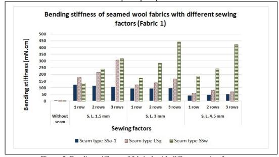
Figure 5: Bending stiffness of fabric 1 with different sewing factors It was found from figure 5 that all sewing factors affected the stiffness of the wool fabrics
