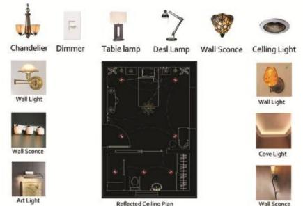
Figure 15: Men's Unit lighting plan & lighting fixtures.
