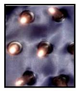
Fig. (42) LEDs passing to the surface through metal grommets
