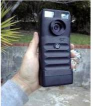
Fig (15) Dycam Model 1 The world's first consumer digital still camera. and optional JPEG compression and serial
