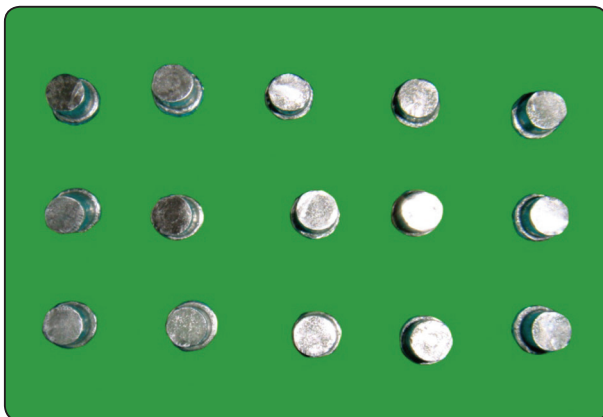
Fig. (3) Part of the metal samples prepared after cleaning and removal of debris.
