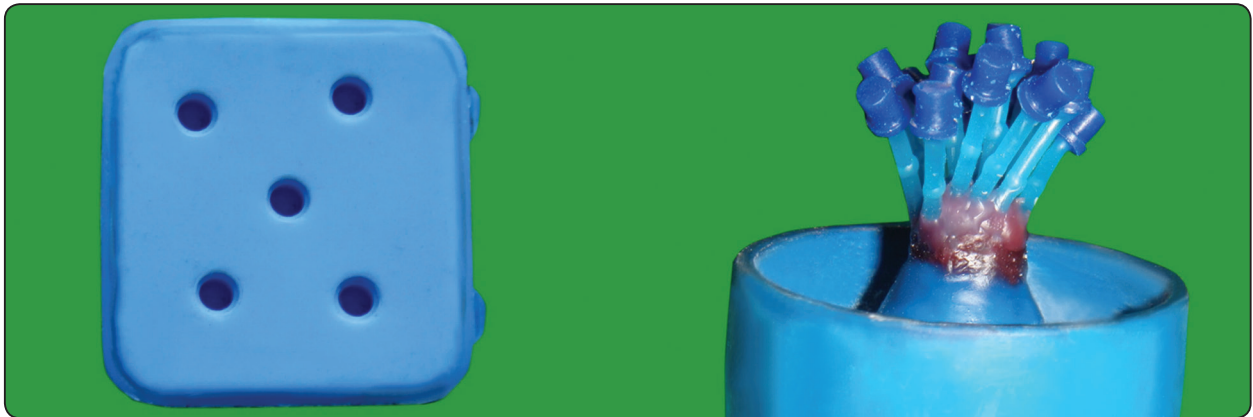
Fig. (2) Mold fabricated to standardize the sample wax pattern, left. Wax patterns of the samples sprued and added to investing ring.
