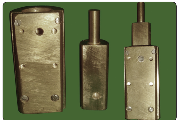
Fig. (6) Disassembled custom fabricated brass apparatus formed by 2 independent pieces, left. Same apparatus after assembling and adding the specimen.
