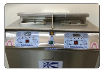
Fig. (3) A custom made Thermocycling machine
