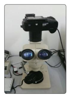
Fig. (5) The stereomicroscope.
